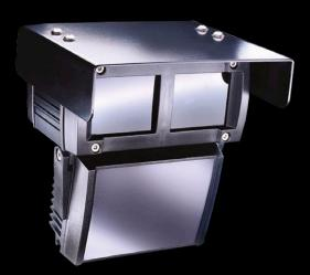
The S-COMM ANPR camera has been designed to accurately and reliably capture number plates for a variety of applications. The cameras, which can be used as stand alone units or in conjunction with the ANPR software, have an impressive 98% image capture rate for legal retroreflective plates. The use of IR LED illumination means that there is no need for regular bulb changes. It also ensures that reliable images can be collected day and night, no matter what the lighting conditions.
