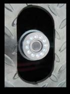
Rated to IP68 the electronics and camera package is water resistant and can be located on virtually any terrain prone to flooding.
